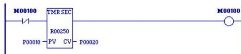
Figure 43: Ladder Logic for Synchronizing Timer
