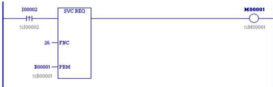
Figure 41: Ladder Logic for Role Switch (SVC_REQ 26)
